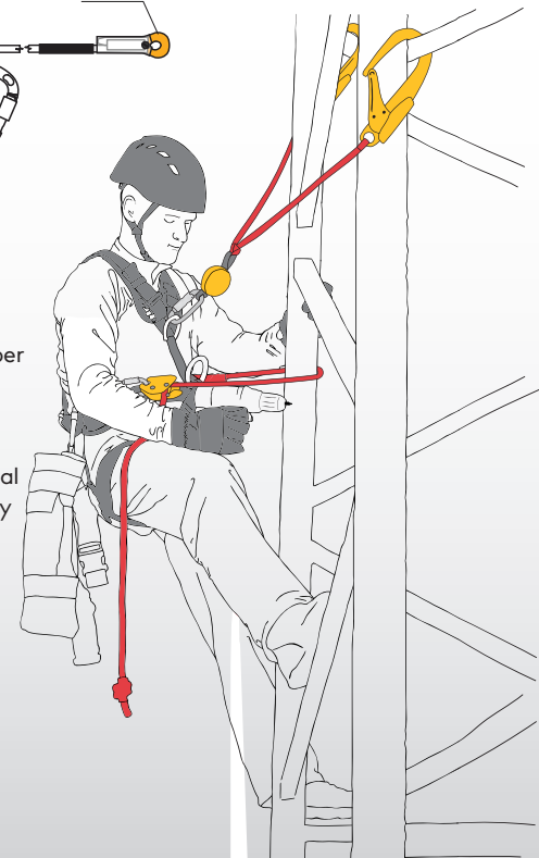
Work positioning on a frame construction
